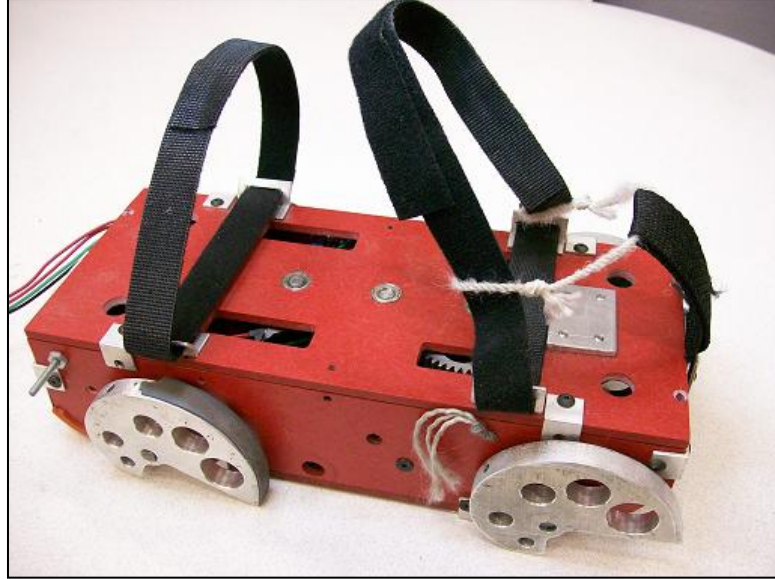
Figure 35: The GEMS straps are designed after traditional sandals
