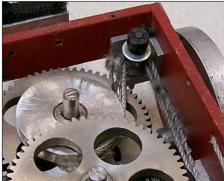
Figure 26: Aluminum reset pulley, redirect pulley, and doubled nylon string
