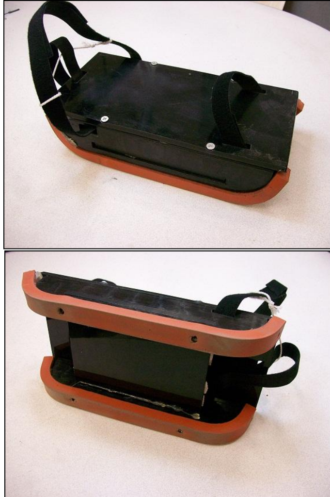
Figure 36: Platform used to compensate for the height of the GEMS
